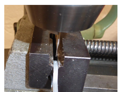
Fig. 15: Clamp both gimbals and drill all 6 D0.5 mm bearings
